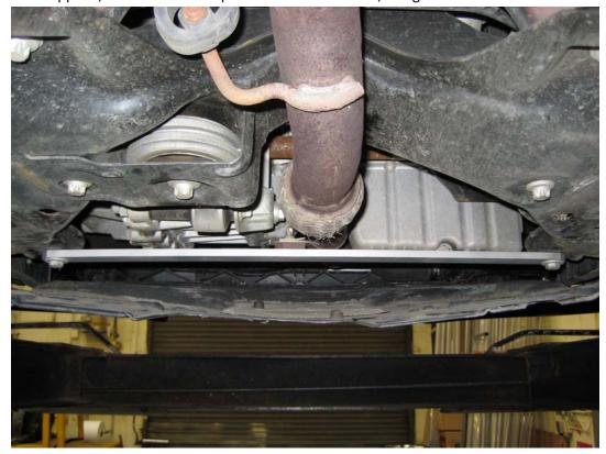
4. Using the supplied 17mm headed bolt, washer and locknut, fix the shorter of the two bars to the rear of the subframe in two unused holes, just in front of the exhaust joiner.
