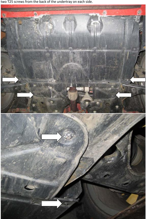
2. With the screws removed, you can pull down the rear of the undertray and expose the thin metal bar the stops the exhaust from hitting the undertray. Remove the two 16mm head bolts and remove the bar.
