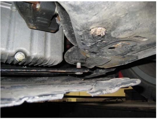
3. The old bar can be discarded, but we will reuse the bolts. Using the longer of the two Forge bars supplied, fix it to the car in place of the old thin bar, using the 16mm bolts.
