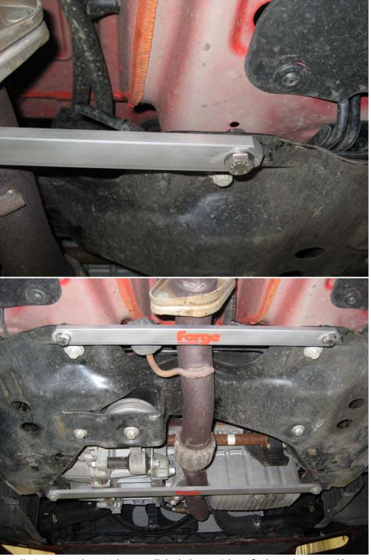
5. Installation is complete. Make sure all the bolts are tight, refit the undertray and lower the car to the ground.
