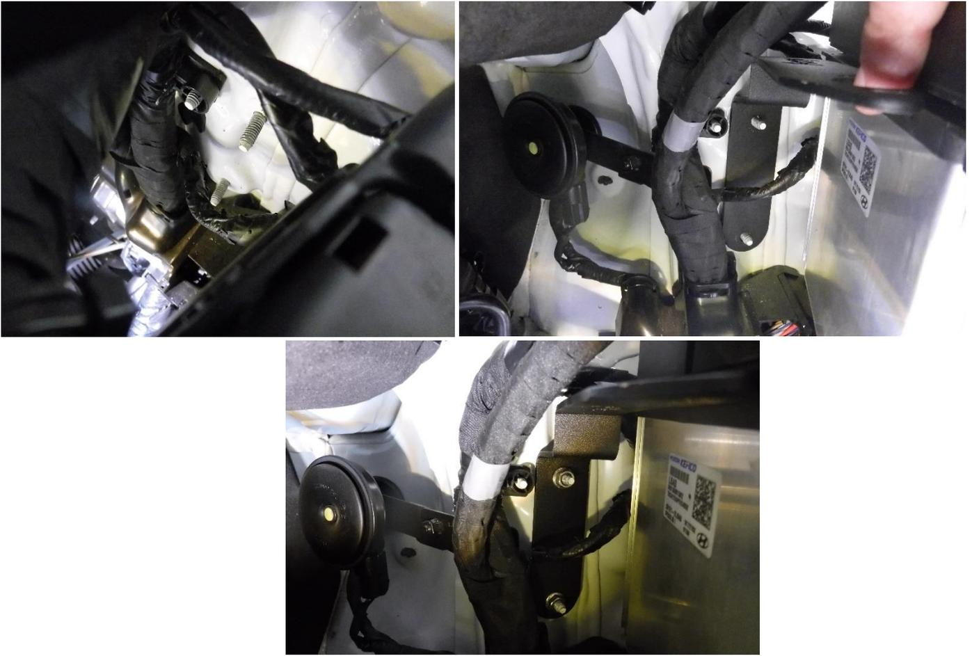
9. Using a 10mm socket and ratchet remove the M8 fastener attaching the oiler breather to the engine. Using pliers or hose clamp removal tool loosen the hose clamp attaching the end of the oil breather hose to PCV. The oil breather hose can now be completely removed.
