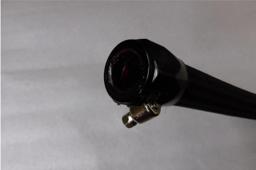
11. Take the AN-8 oil hose (smaller diameter) from the FMOC10 Kit and fit it to the OEM turbo adaptor. Re-install the turbo adaptor with the oil line fitted. Make sure the O-ring is in place when fitting.
