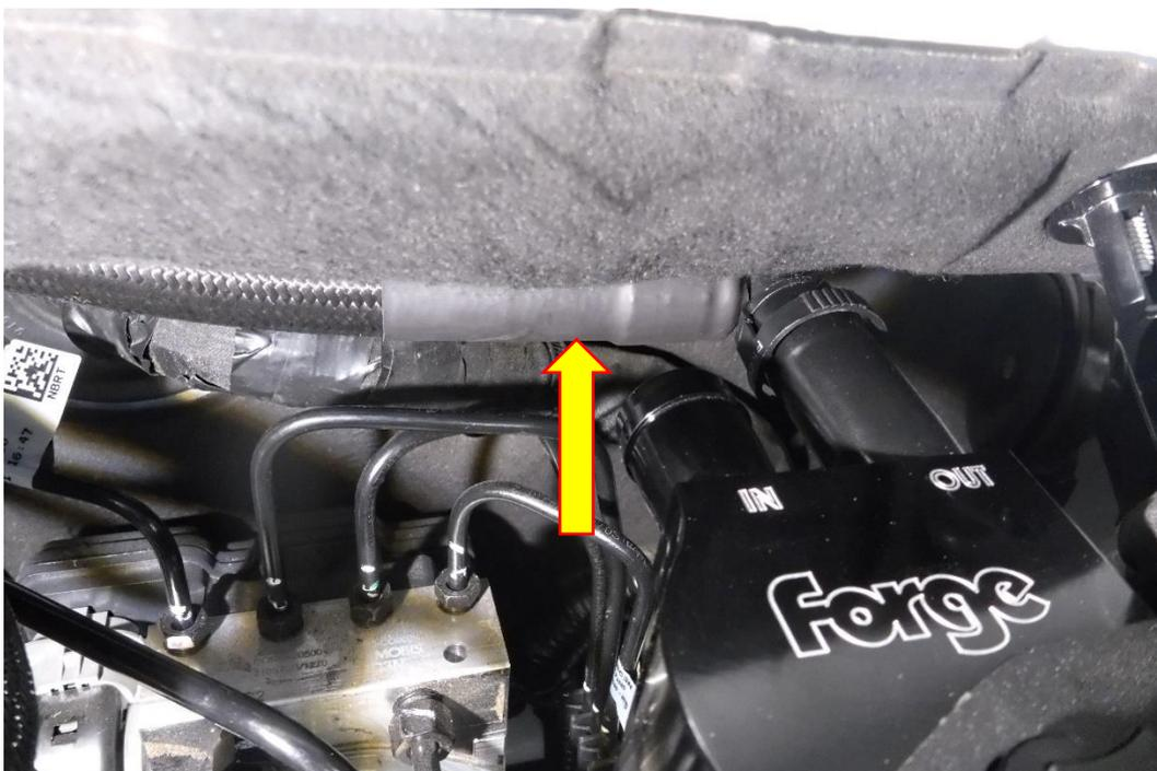
14. Using the large cable tie from the FMOC10 kit secure the fitted oil line to the coolant pipe below it. Using a 7mm socket and ratchet secure the hose clamp on the oil line. Re-fit the actuator wiring loom.
