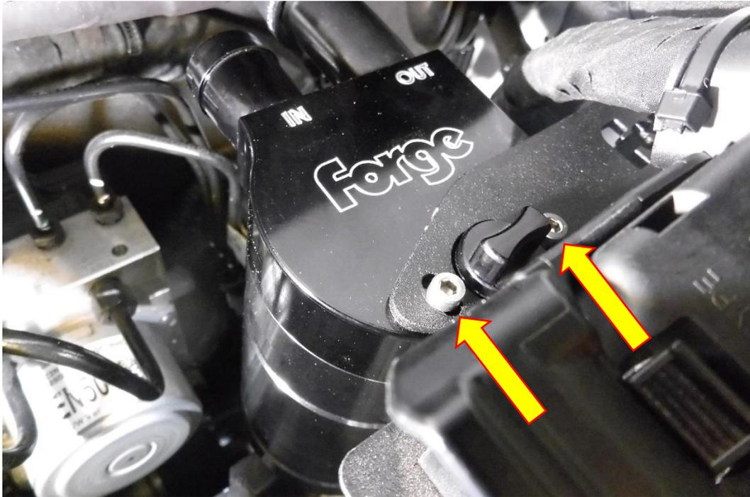
13. Attach the fitted oil line to the **OUT** port of the catch can, push the plastic fitting until you hear it click.
