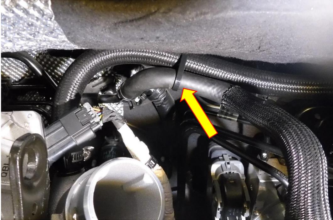
15. Fit the remaining oil line, the plastic end to the IN port of the catch can and the other end to the vehicles PCV. Using a 7mm socket and ratchet secure the hose clamp of the oil line.
